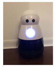
**Figure 3:** Kuri is a small social robot. It's interaction involves autonomous or app controlled movement, expressive eyes, babbling sounds, and a heart light that produces different colours.
